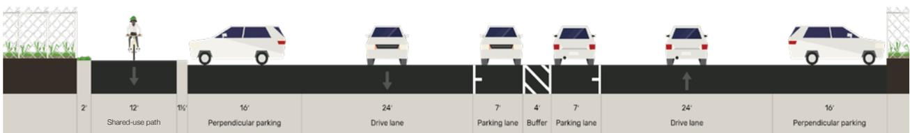
FIGURE 18: MBTA Orient Heights Preliminary Proposed Cross Section with Limit of Work Pushed to Property Line (facing west)
